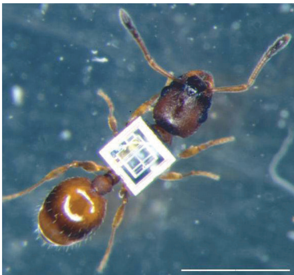
Figure 1. Radio-tagged Temnothorax albipennis worker. Scale bar 1mm. Photograph by Nigel Franks.
