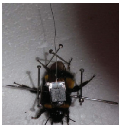
Figure 4. Showing a mock up of an IFF transponder tag on a Bombus terrestris dalmatinus forager (left) and detail of a VHF radio transmitter on a dragonfly ( Aeshna sp.) (right).
