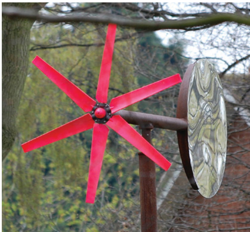
Figure 4. Microturbine with red rotor blades. Simple changes like this to the colour of a turbine may help to reduce insect attraction to the structures.
