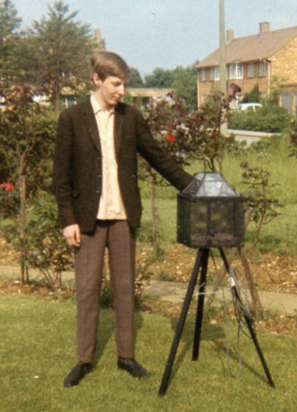
HDL with his home-made Williams-design tungsten filament light trap which he made and used in 1968 to collect moths prior to actually getting a job at Rothamsted in July, 1969. Photo: Front garden of family home, Adeyfield, Hemel Hempstead, probably taken by HDL's mother, Phyllis M. Loxdale.
