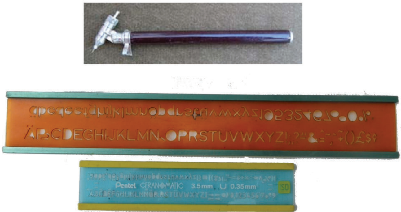
Fig. 1. Above, pen with tubular nib for use with below, plastic stencils (photo of pen courtesy of David Riches).
