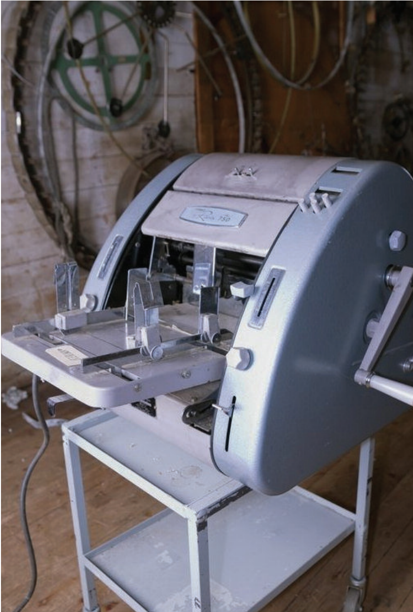
Fig. 5. A Roneo duplicator (photo courtesy of the Museum Centre in Hordaland, Norway).
