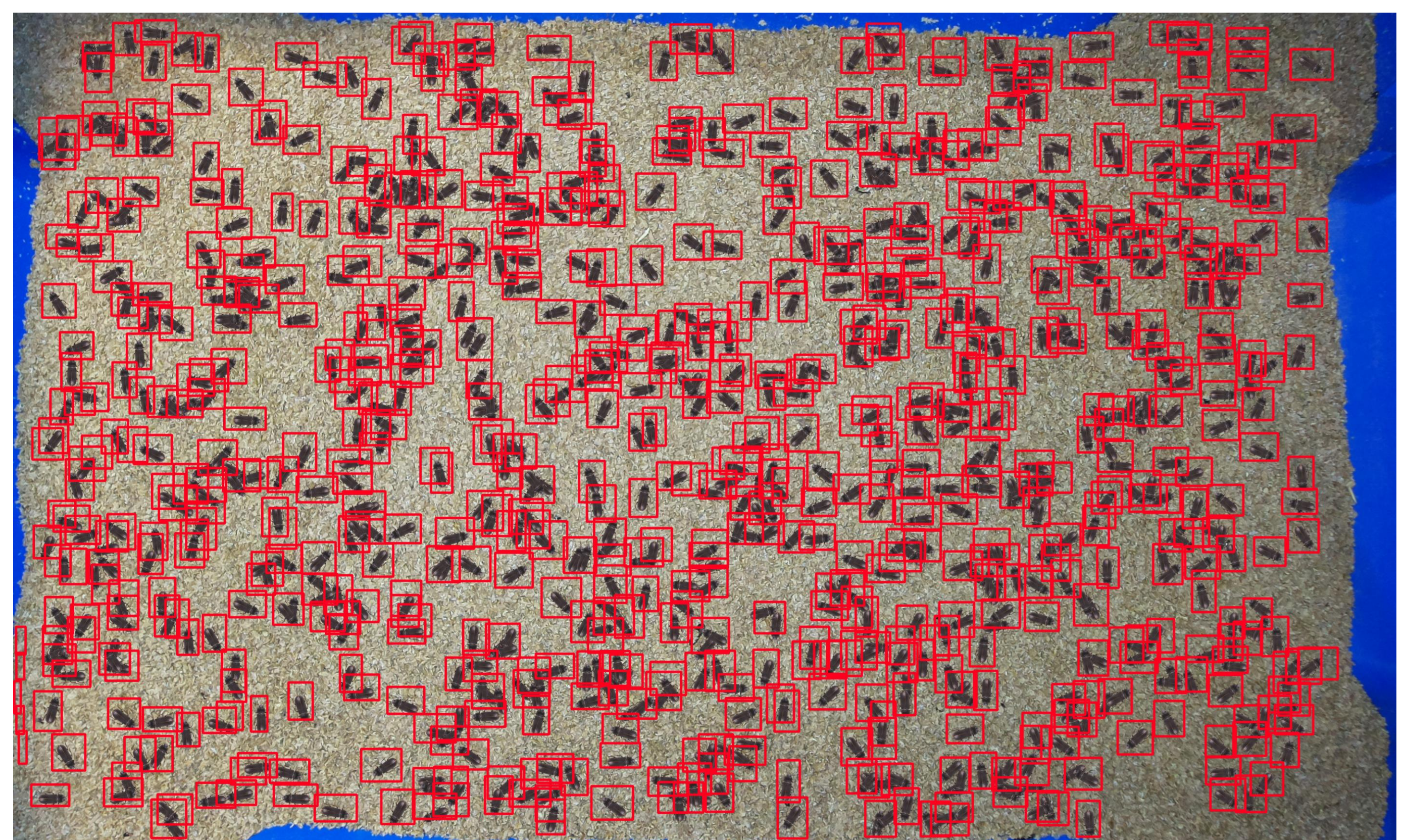
Detection using YOLO (500 to 1000 adult mealworm beetles in single tray)
