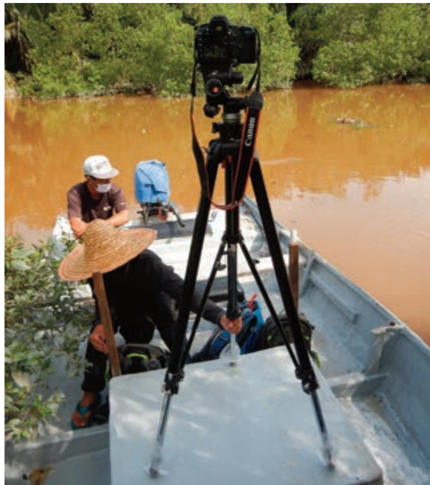
Figure 3. Camera and tripod set up on a raised platform in the boat. During photography, the frontal tripod leg is held down firmly as shown.
