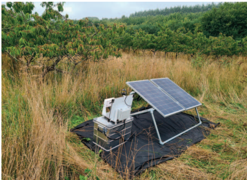
Fig. 1. System for attracting and photographing moths (credit Grace Skinner).
